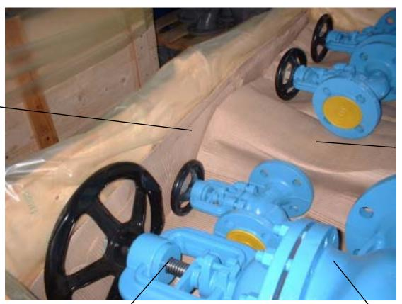
Corrugated cardboard separators used as cushioning can be a significant source of corrosion.
